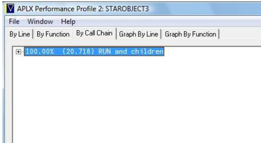
This shows that, unsurprisingly, 100% of the time was spent in our top-level function RUN and in all the functions called by it. We can now use the twist-downs to drill down into the hierarchies of calls to see how that time was divided up:
